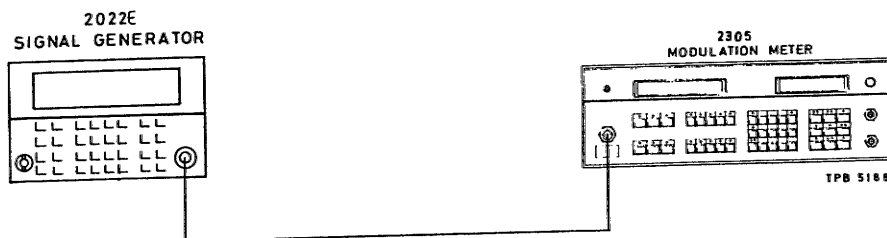
Fig. 5-7 Test gear arrangement to check AM depth and distortion
