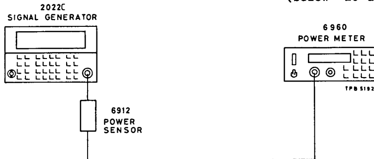
Fig. 5-3 Test gear arrangement to check RF output
