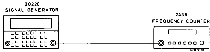
Fig. 5-2 Test gear arrangement to check frequency accuracy
