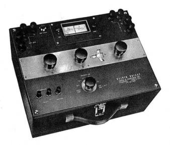
A portable bridge for precision measurements and calibration of meters, components, windings and other instruments.
