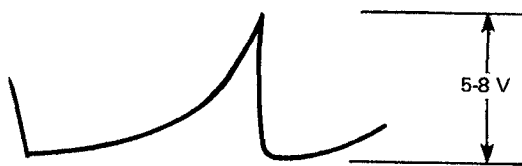
Figure 6-4. TP-6 Waveform With RATE Control Fully Clockwise
