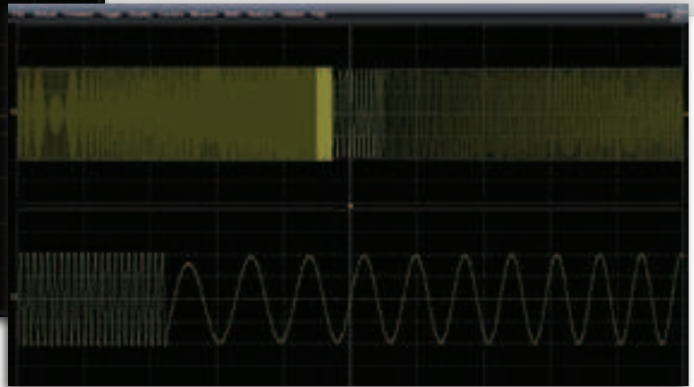
Capture up to 30 seconds of data at sample rates as high as 10 MS/s for trending and searching for events.
