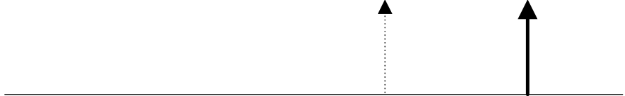
Figure 8-8. Interval Trigger that triggers when the interval falls within the selected range: T1=range's lower time limit; T2=range's upper limit. The broken upward pointing arrow indicates a potential trigger, while the bold one indicates where the actual trigger occurs — on the positive edge within the selected range.
