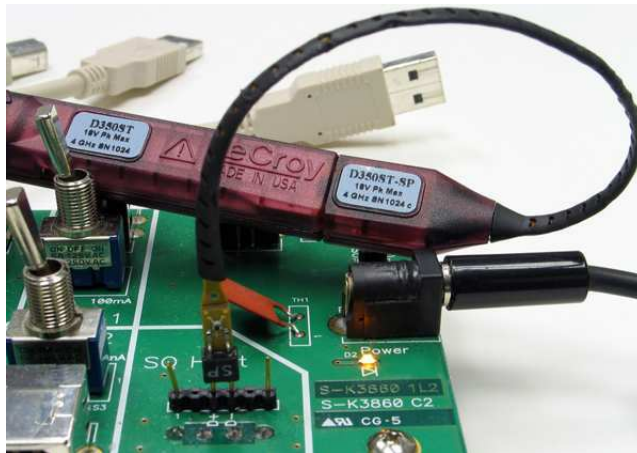
D350ST-SP Differential Probe Connected to the Test Fixture
