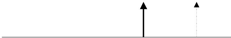
Figure 8–11. Interval Trigger: Trigger if the interval is greater than the selected width.
