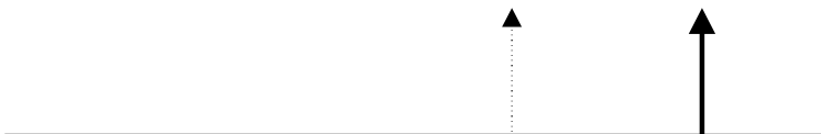
Figure 8–10. Interval Trigger: Trigger if the interval is smaller than the selected interval.
