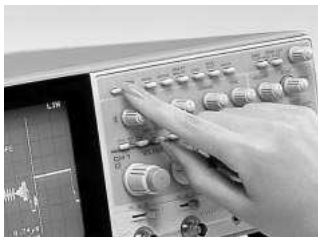
Switching between the real mode and the storage mode can be performed with the single press of a button.
