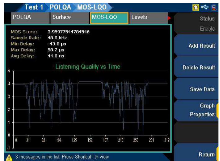
Figure 7. The MOS (Mean Opinion Score) scoring, indicating the rating of the DUT's voice quality.
