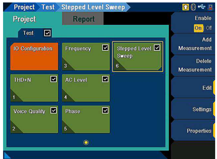
Figure 9. The test sequence control function comes with a selection of preconfigured measurements and allows users to select the most frequently used test sequences for their daily measurement.
