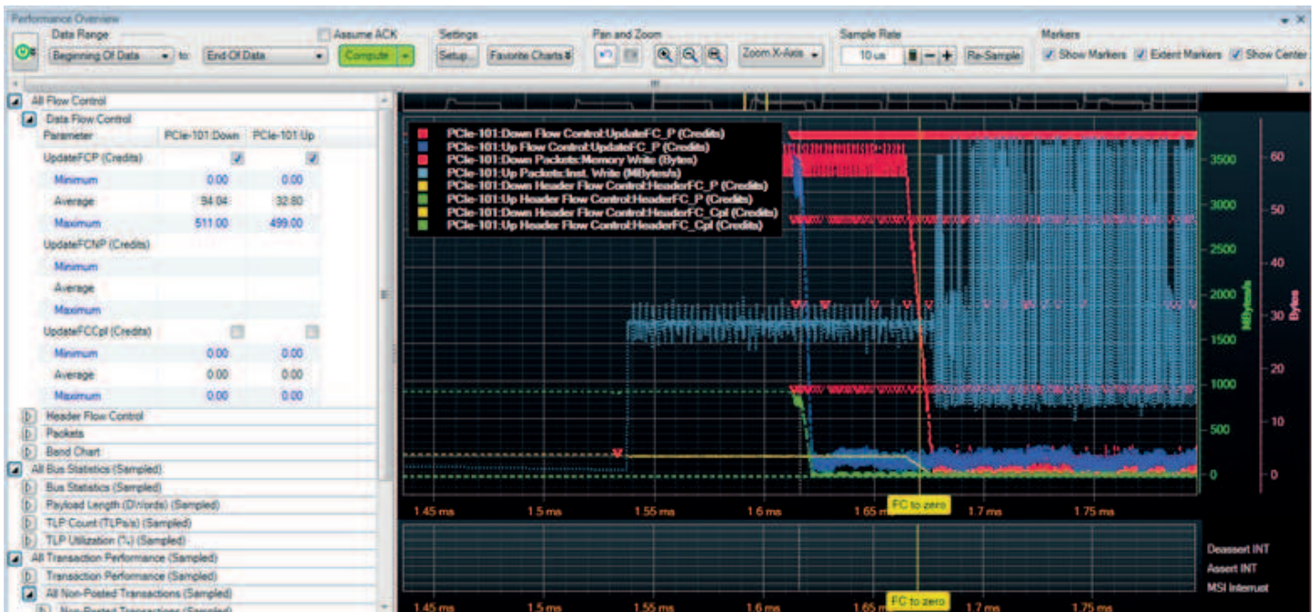
Figure 16. Easily identify credit exhaustion with flow control analysis for data and header flow control analysis.
