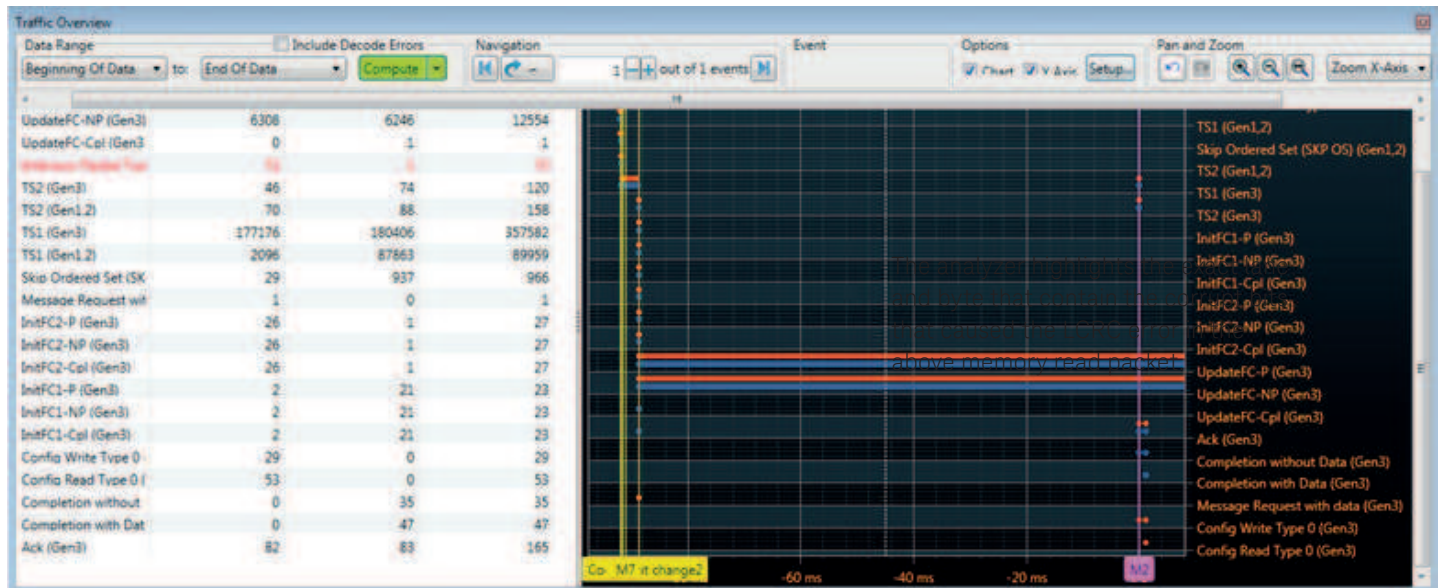
Figure 4. The Traffic Overview shows all of the packets in the capture buffer in a time scale display. Instantly access to any packet by clicking on the graph.
