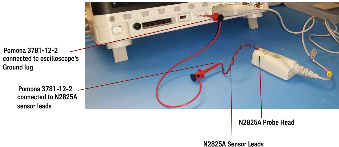
Figure 33 Probe Calibration Terminals Connections on an InfiniiVision-Series Oscilloscope
