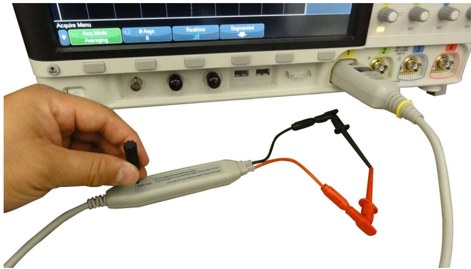
Figure 7 Adjusting the Offset Using the Supplied Tool
