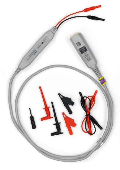
Figure 1. N2804A 300-MHz differential probe with standard accessories.
