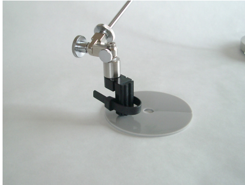
Figure 11 The universal holder placed on the probe rest
