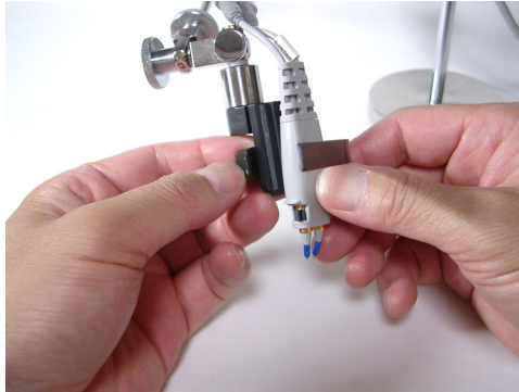
Figure 3 Probe aligned with rubber ribs
