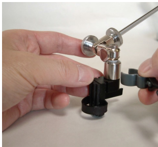
Figure 10 Attaching the magnifying glass
