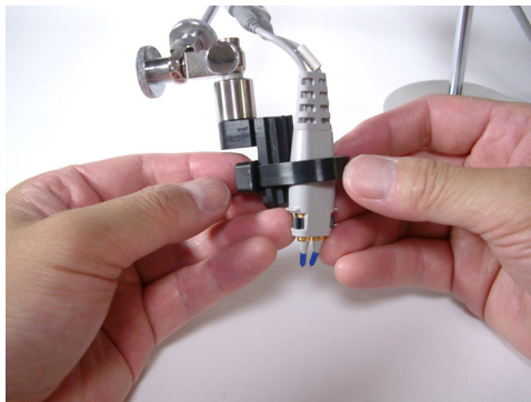
Figure 4 Probe tie wrapped around the probe
