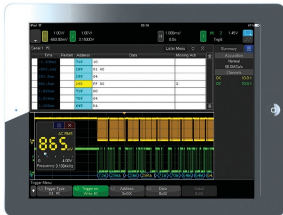
Figure 37. Tablet virtual front panel control.
