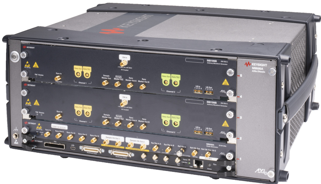
Figure 7 Typical configuration of the M8199B AWG with M8008A Clock Gen.
