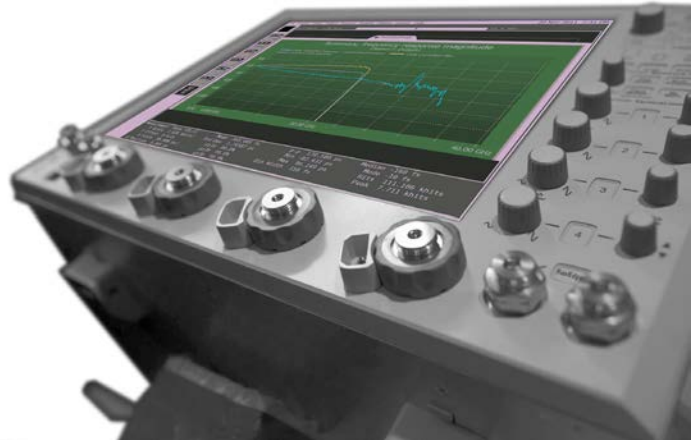
PrecisionProbe software characterizes cables to 63 GHz
