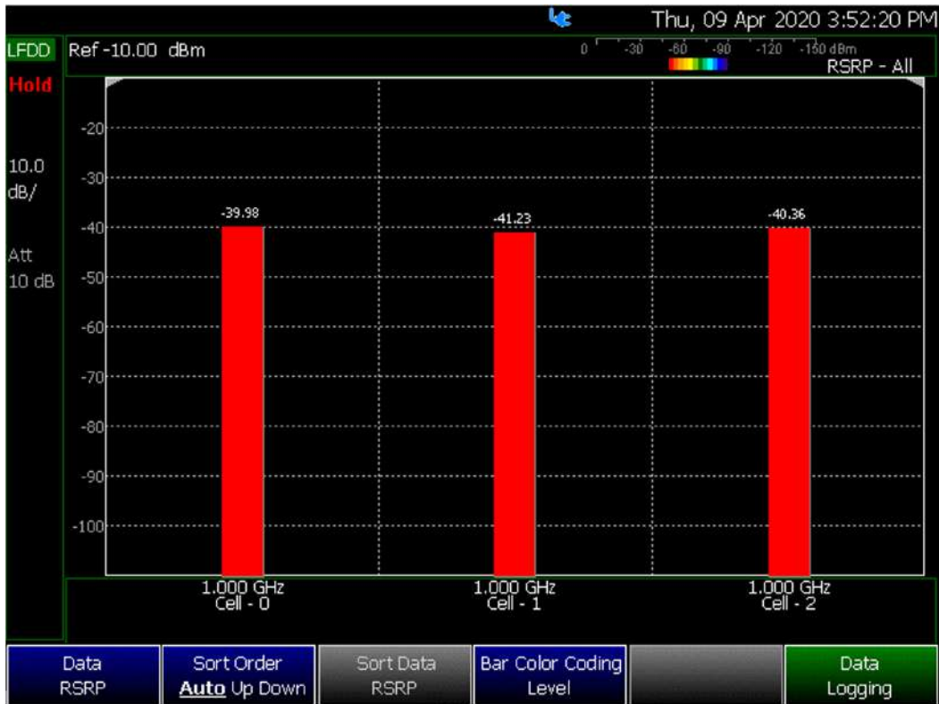
Figure 13-4 LTE FDD Bar Chart – Level Example
