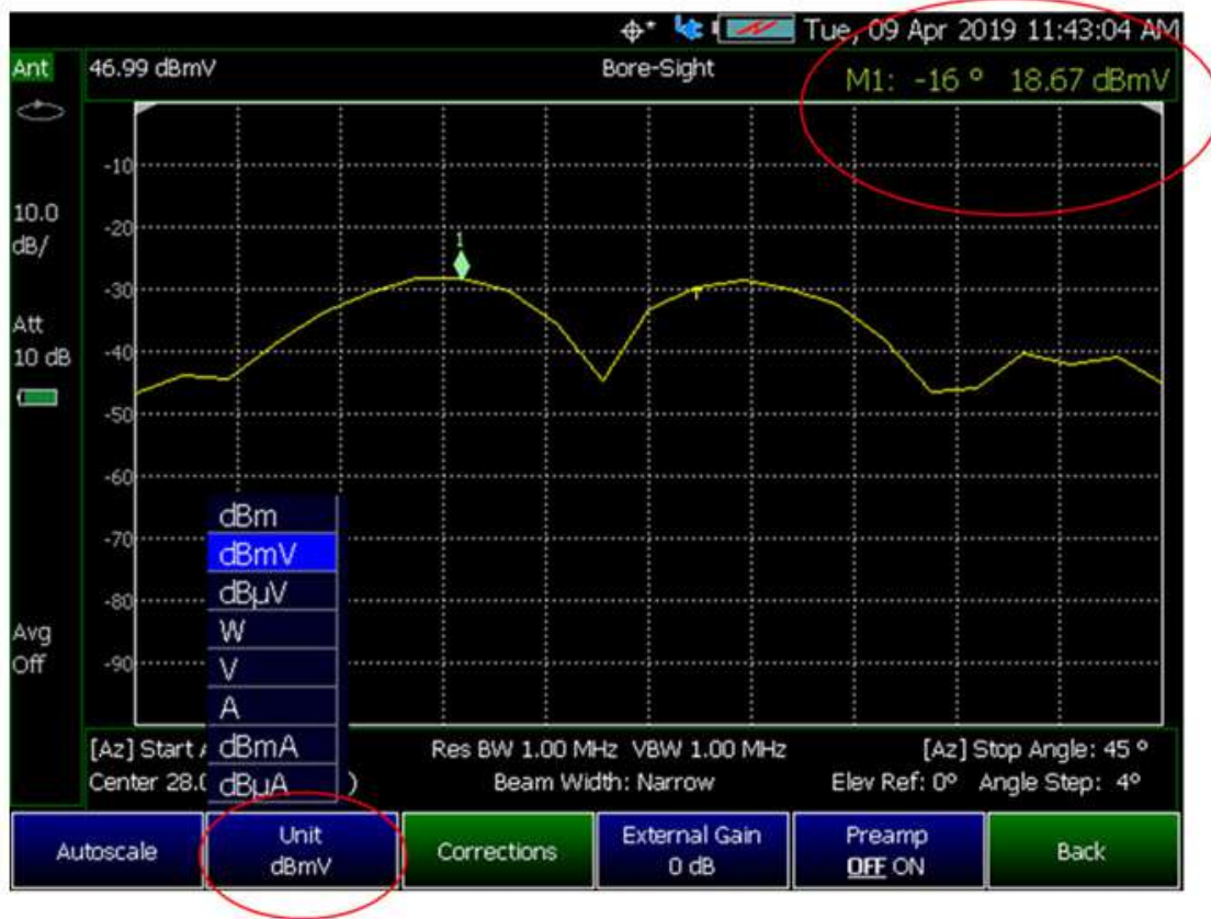
Figure 14-18 Field Strength Annotation that can be Logged and Played Back
