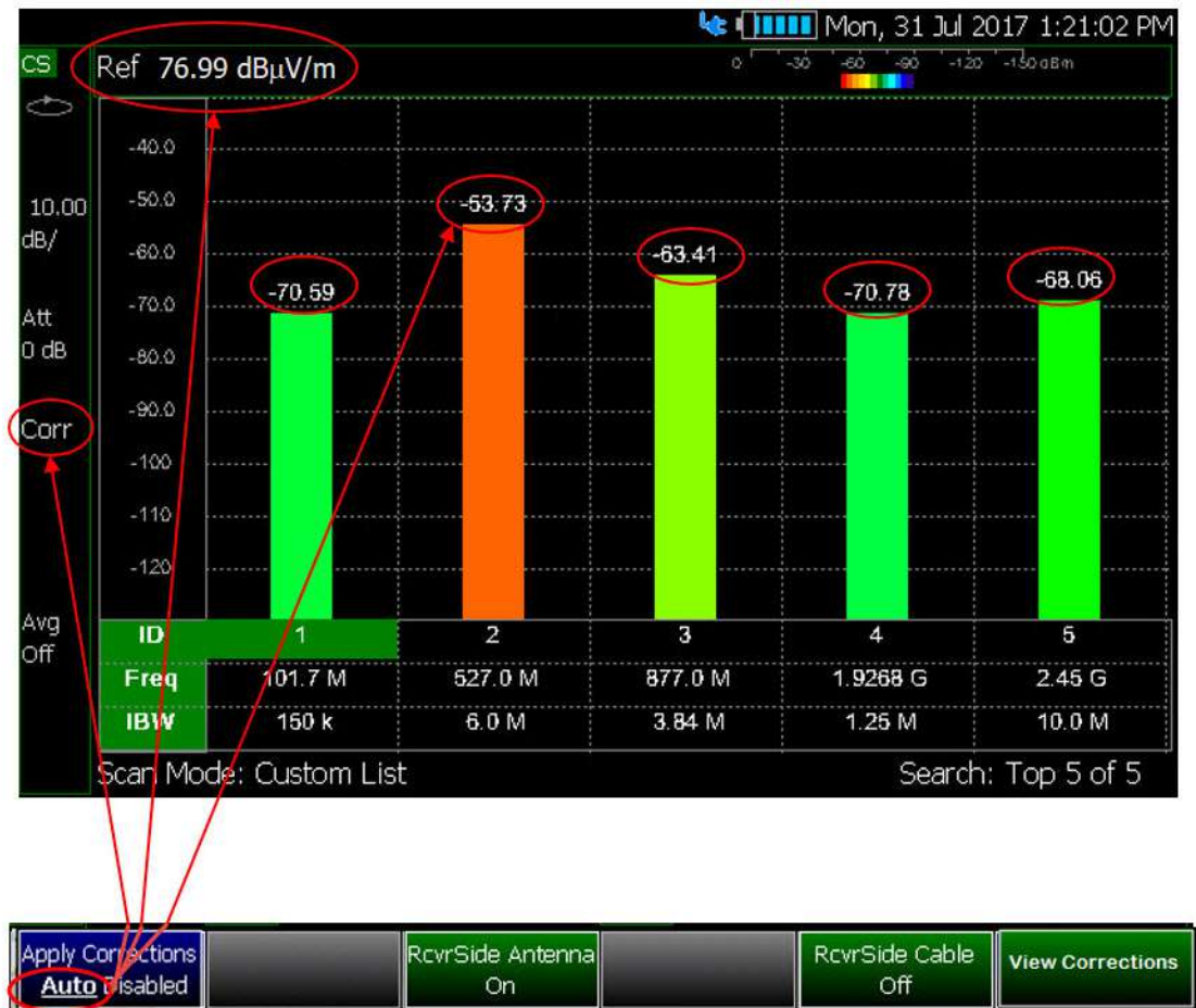
Figure 28-18 Apply Corrections Set to Auto
