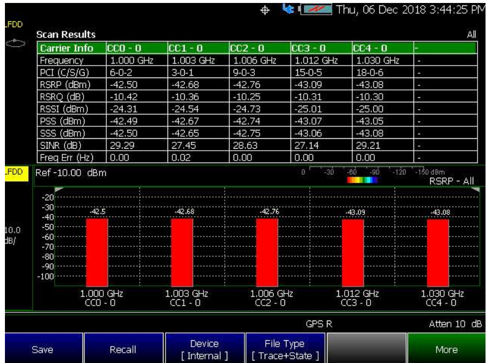
Figure 13-21 Example of LTE FDD with Multiple Carriers, Single Cell Site, and KPI's
