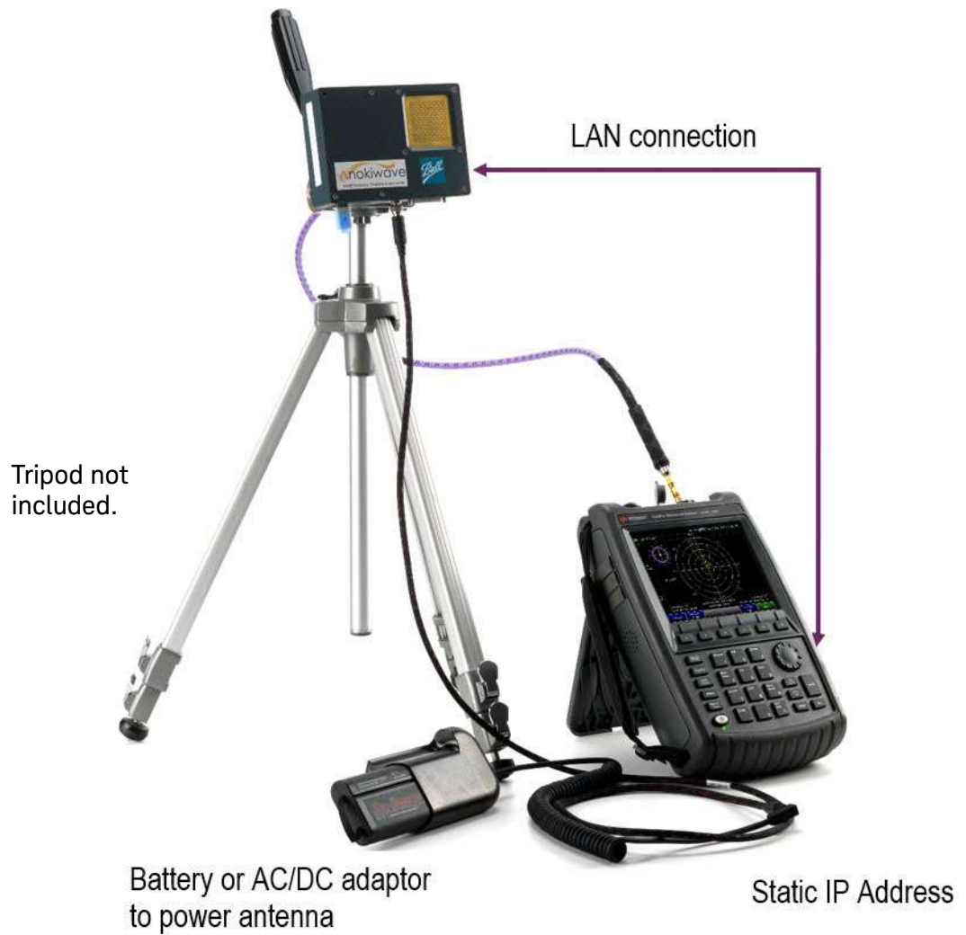
Figure 14-1 Example of local point-to-point LAN connection
