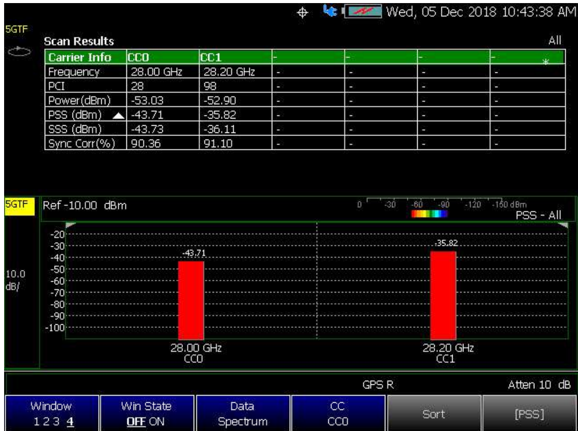
Figure 13-14 Example of 5G TF Single Carrier and Single Cell
