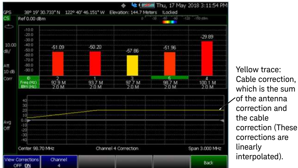
Figure 28-17 Yellow Trace with Cable and Antenna Corrections
