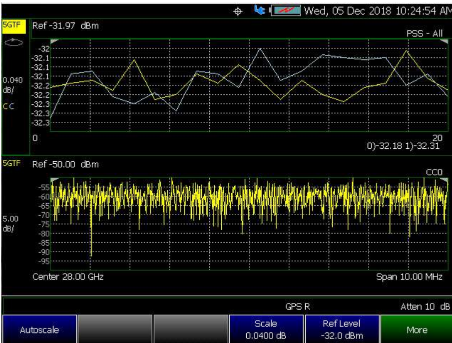
Figure 13-25 Spectrum and Strip Chart Display Type – 5G TF
