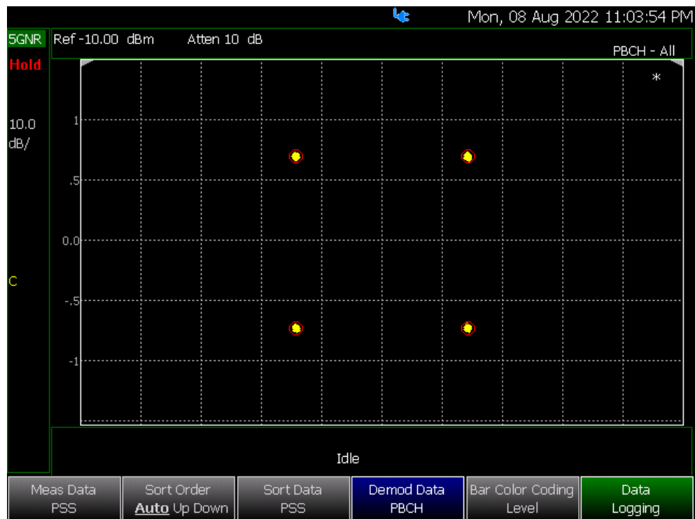
Figure 13-11 5G NR EVM Constellation Example – Measure Data set to PBCH
