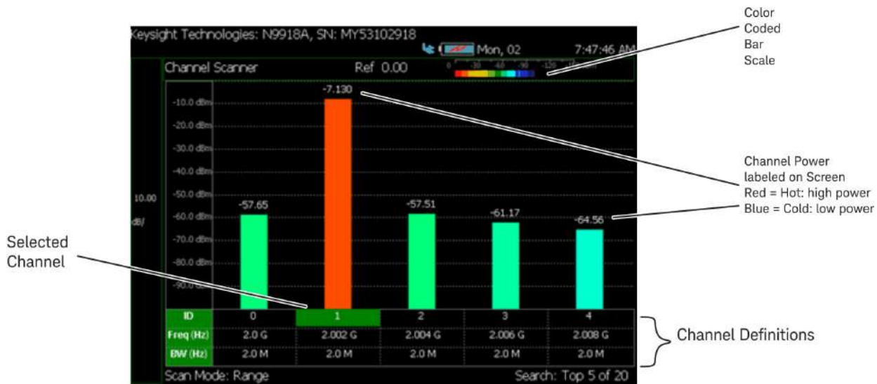
Figure 28-1 Display Example: Measure 5 Channels Spaced 2 MHz Apart
