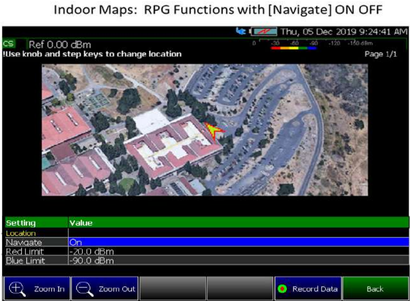
Figure 16-3 Using Mapping (Option 352) - Satellite View for Indoor Mapping
