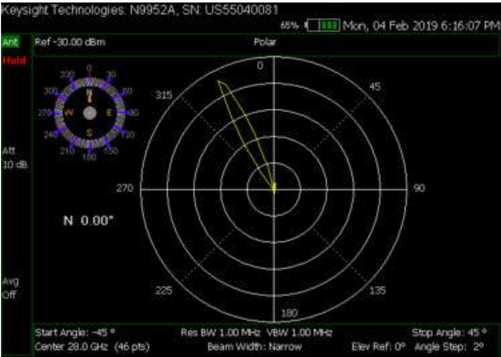
Figure 14-3 Polar Scan with compass displayed
