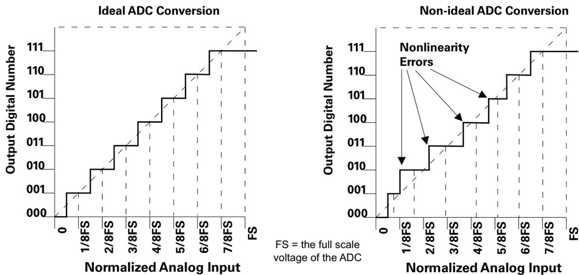
**Figure 8** ADC Non-linearity Errors for a 3-bit ADC
