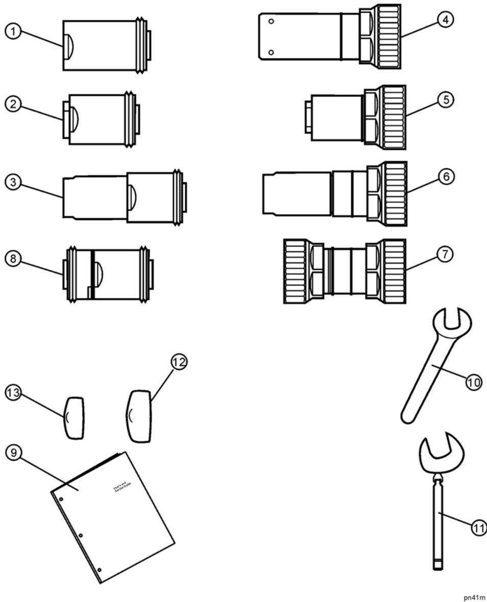
**Table 6-1 Replaceable Parts for the 85038A/F/M Calibration Kits**
