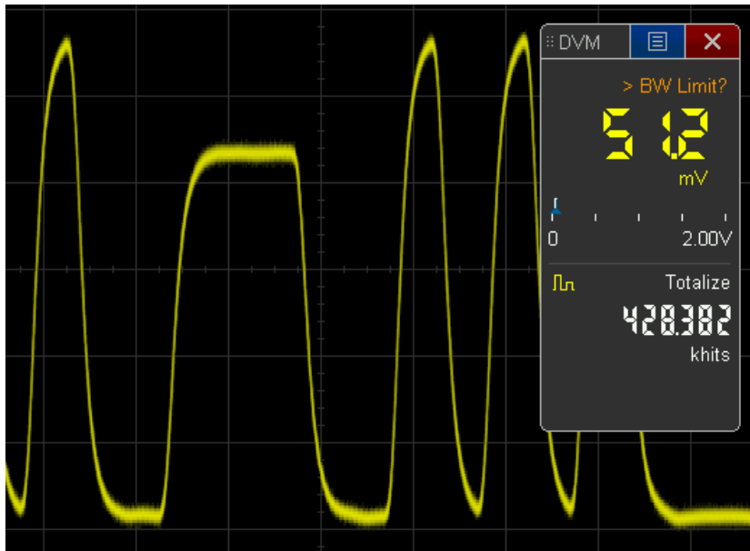
Figure 35. Totalizing the number of runt errors.
