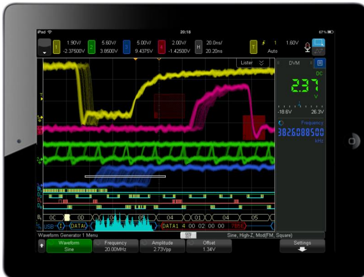
Figure 53. Controlling the 6000 X-Series via tablet device.
