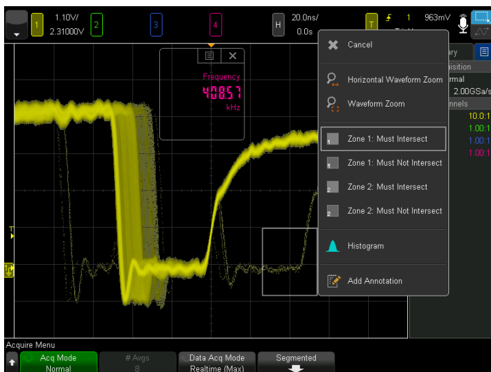
Figure 11. Draw a zone (box) around the anomaly.
