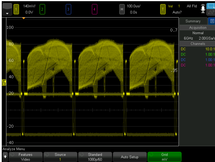
Figure 45. Triggering on a 1080p/60 signal.
