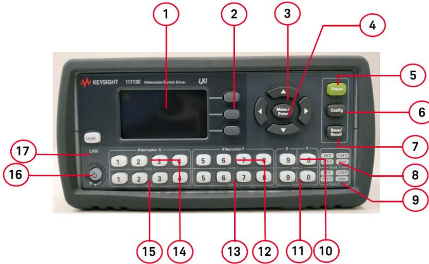
**Figure 1-3** 11713E front panel features
