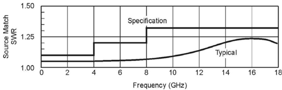
**Figure 1** Leveling or ratio measurement source match graph
