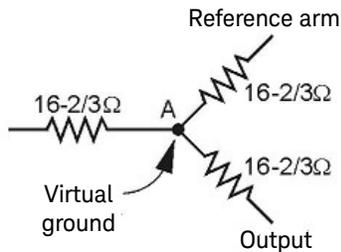
**Figure 4** Three-resistor power splitter
