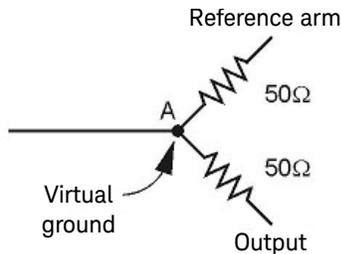
**Figure 5** 11667A power splitter schematic
