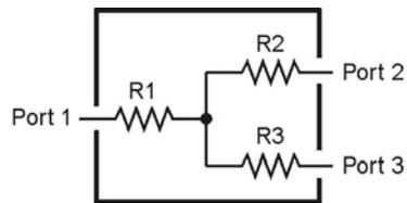
**Figure 2** Typical power splitter diagram
