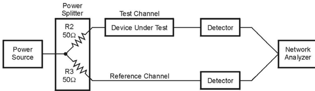
**Figure 3** Simplified diagram of a network analyzer system
