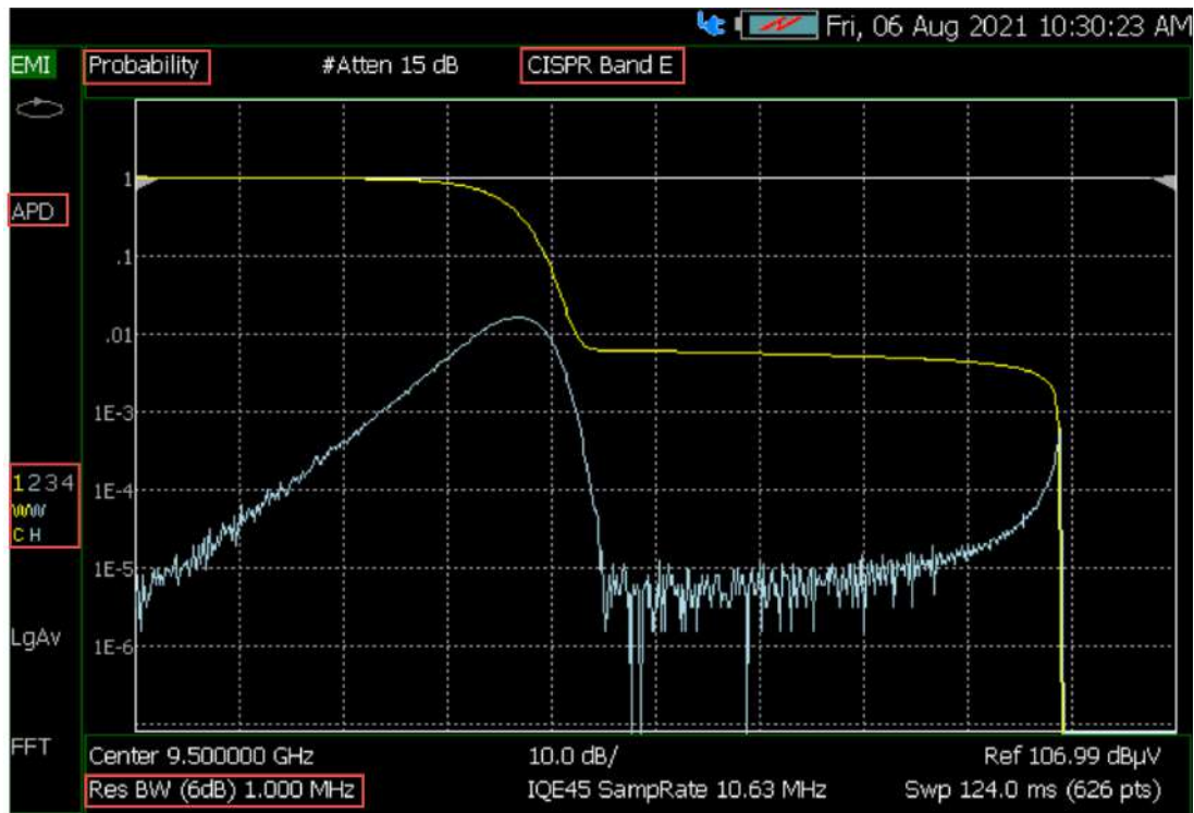
Figure 12-5 APD Statistics Example 2 – CW
