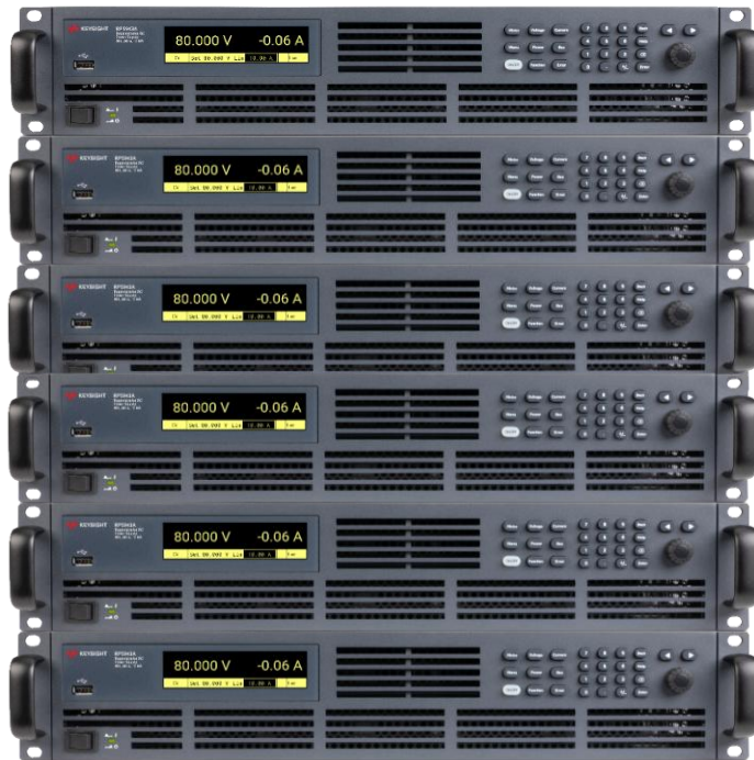
Figure 3. Parallel operation for more power
