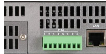
Figure 4. Digital control port on the rear panel
