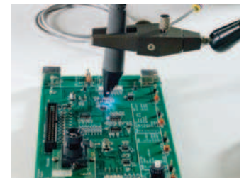
N2795A/96A comes with a headlight for better visibility while probing
