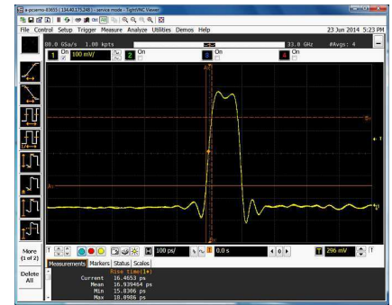
Figure 5. 100 ps pulse with 17 ps risetime.
