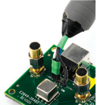
N2750A with N4822A socketed tip for application fixtures
