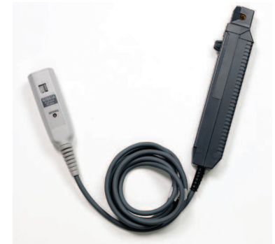
N2893A 100-MHz current probe with AutoProbe interface
