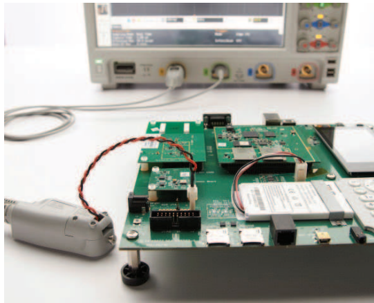
N2820A high-sensitivity 2-channel current probe
