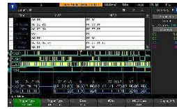
Figure 18. SPI 4wire decode and trigger.
