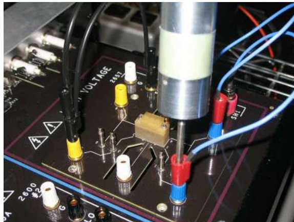
Figure 45: 8020-DP contacting 8010 SHI terminal
