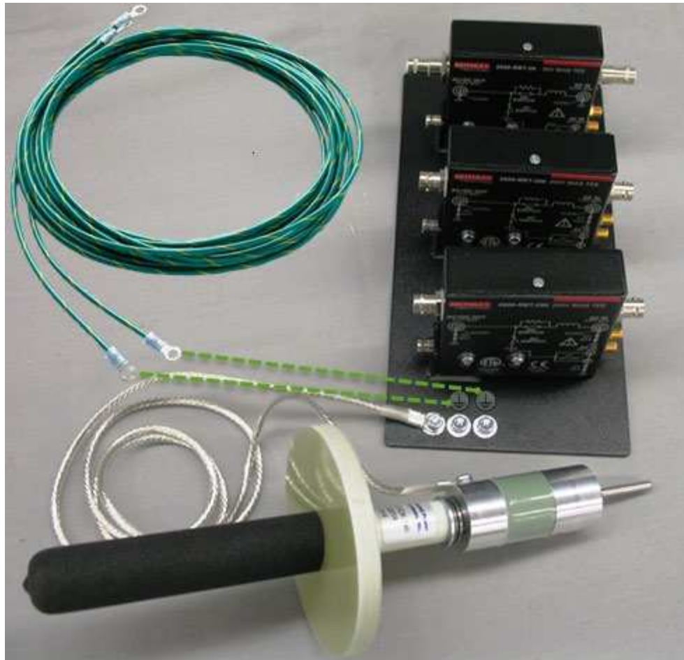
Figure 43: 8020-DP connected to bias tee bracket ground
