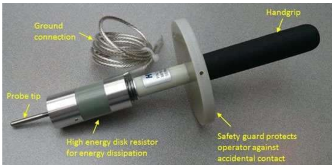
Figure 40: 8020-DP High Voltage Discharge Probe
