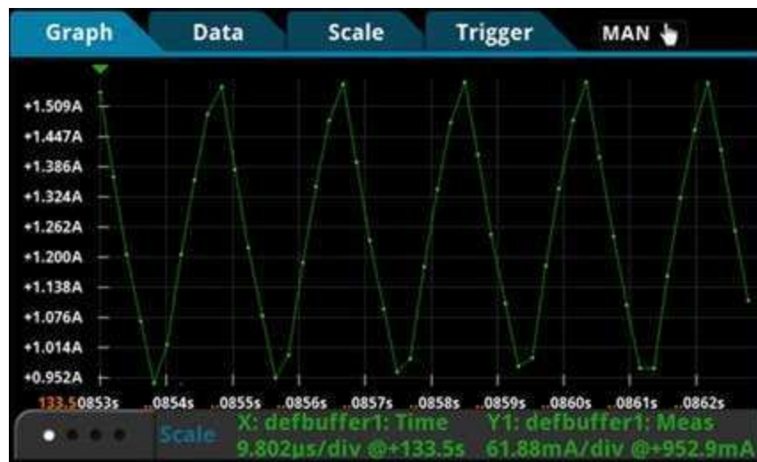
Figure 42: Inductor current linearity results at 4 ohms
