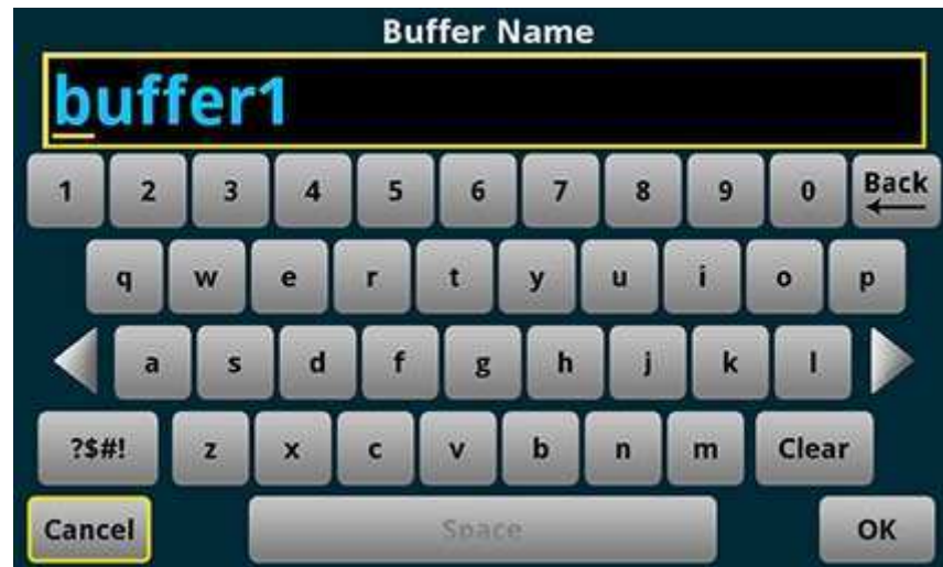
Figure 3: DAQ6510 front-panel keyboard for information entry
