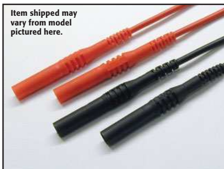
Model 8607 1kV Source Banana Cable Set: The 8607 cable set is made up of one red and one black high voltage test lead with fixed safety banana plug ends. The leads are 1 meter (3.3 ft) long and have a voltage rating of 1500V DC.
