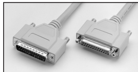
CA-126-1 Digital I/O Cable: 1.5m (5 ft) of cable, from DB25 male to DB25 female.
