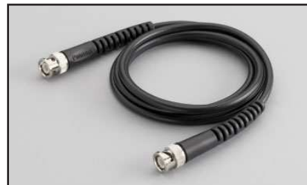
Model CA-19-2: 1.5m (5 ft) RG58 cable terminated with a BNC male plug on each end.
