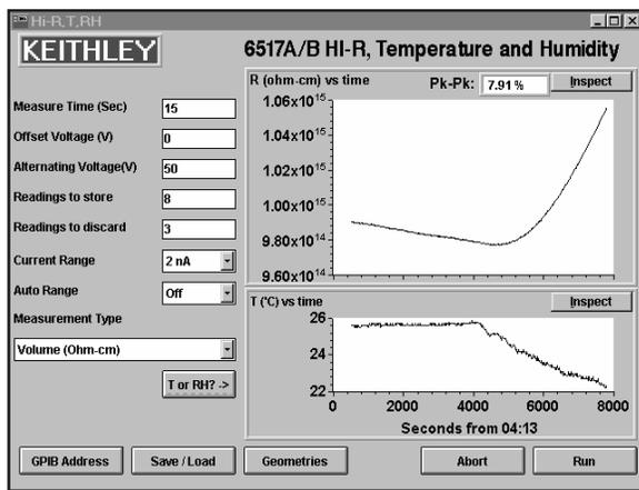
The Model 65 package can eliminate drift and noise in difficult materials, so it is possible to determine characteristics of the material that were previously obscured, such as temperature coefficient. The Model 6524 software allows graphing resistance/resistivity plus temperature or humidity vs. time on the same screen. This makes it easy to observe and calculate the dependence of a sample's resistance/resistivity vs. temperature and humidity.
