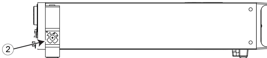
Figure 8: Remove mounting ears
