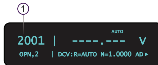
Figure 7: Select a channel from the Series 3700A front panel
