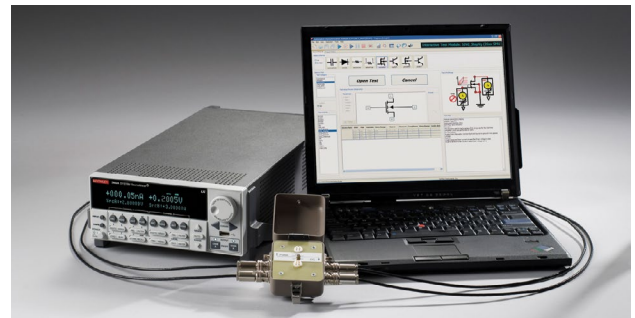
The flexible software architecture of ACS Basic Edition allows configuring systems with a wide range of controllers and test fixtures, as well as the exact number of SourceMeter SMU instruments the application requires.
