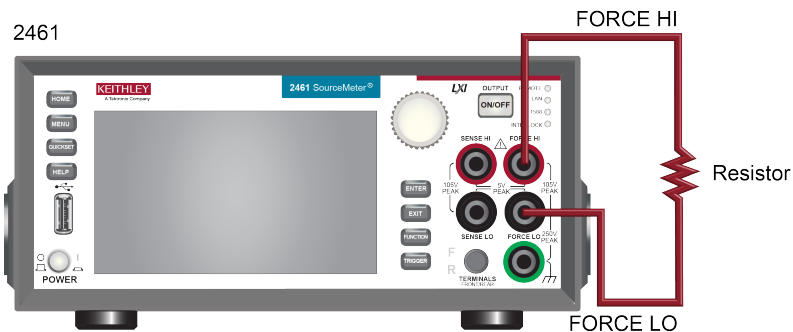
Figure 19: Model 2461 2-wire front-panel connections
