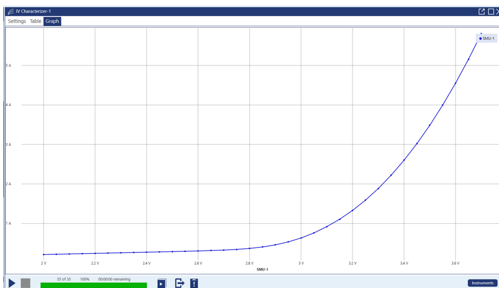
Figure 39: Results of running an I-V sweep on a high-brightness LED
