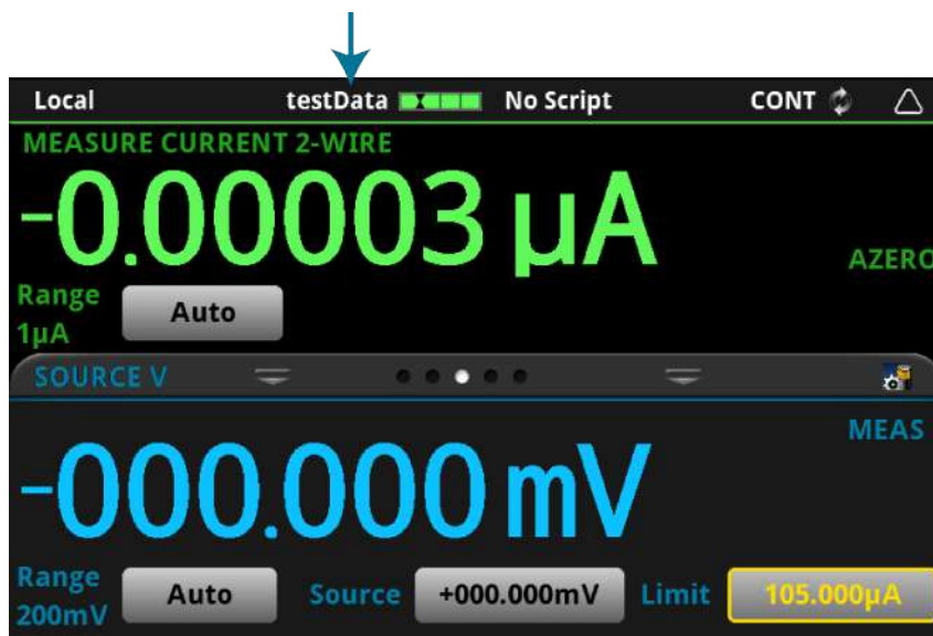
Figure 125: Active buffer indicator
