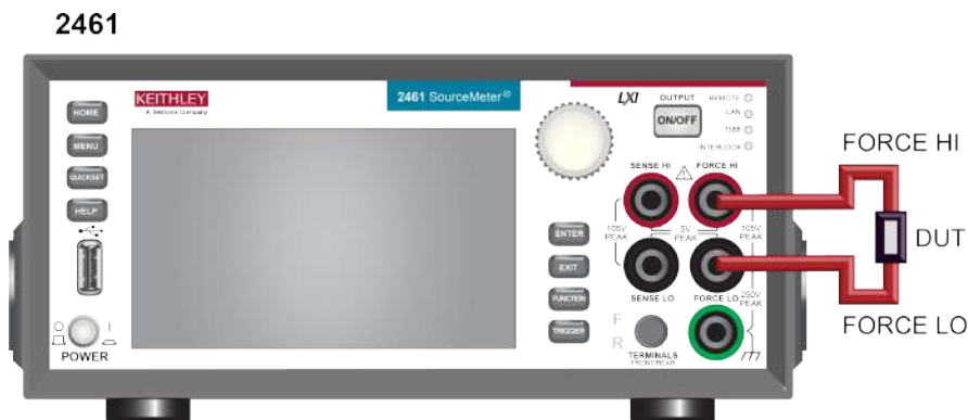
Figure 59: 2461 2-wire rear-panel connections
