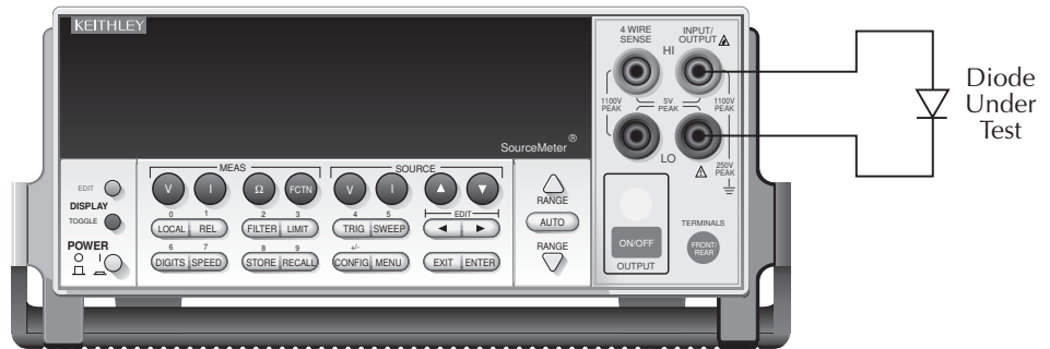
Figure 10-8 Connections for diode I-V tests
