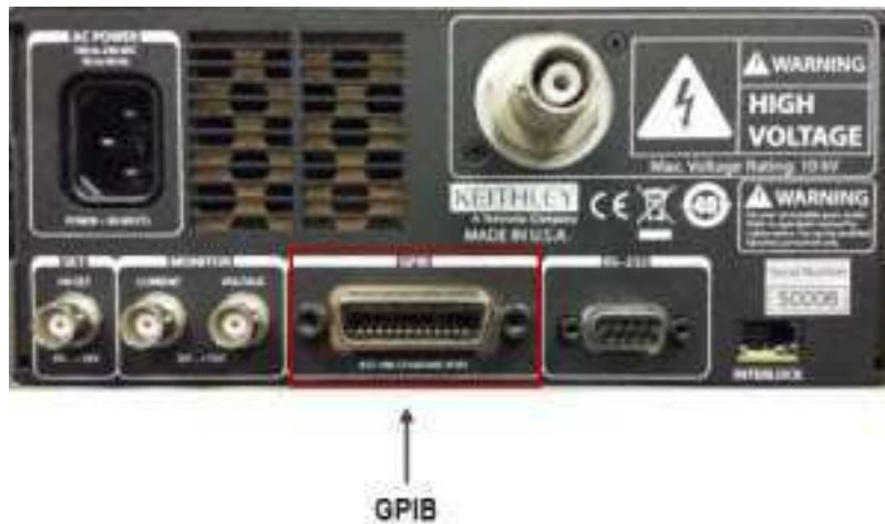
Figure 9: Model 2290-10 rear panel GPIB location
