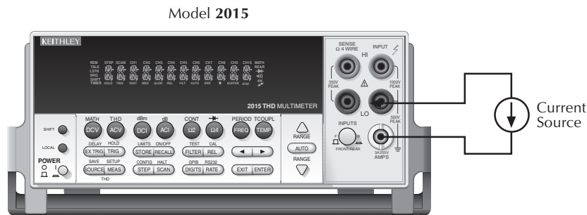
Figure 2-5 DC and AC current measurements
