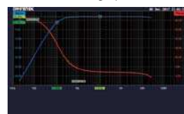
Cursor measurement for the determination at 3dB cut-off frequency of the high-pass filter.
