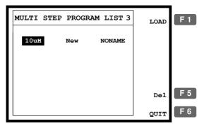
3. Use the arrow key to move the cursor to the program to be recalled (loaded).
