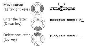
3. Press the Enter key to confirm the file name. To quit the new program mode, press the Clear key.
