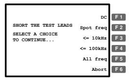
4. Always select F5 (All freq) when using the standard fixture set included in the LCR-8000G package.
