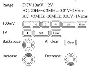
When the entered value does not fit in the range, the LCR-8000G automatically selects the nearest value.
