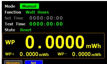
5. Press **Enter** button to enter **Mode** item. Use up and down arrow keys to toggle between Manual and Standard mode. Press Enter button again to confirm your selection.
