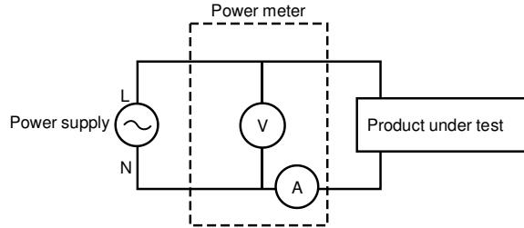
$$\text{Power loss} = (\text{Input current}[A])^2 \times 500\text{m}\Omega$$
