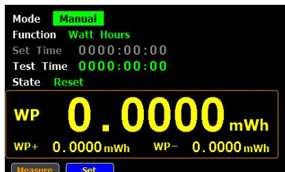
If you select standard mode, you need to set integrator measurement time before using integrator function. It can be set from 1 second to 9999 hours, 59 minutes and 59 seconds.
