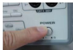
4. The display turns on and shows the last function that was used before the power was reset.
