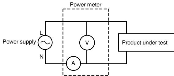
$$\text{Power loss} = (\text{Input voltage[V]})^2 / 2.4M\Omega$$
