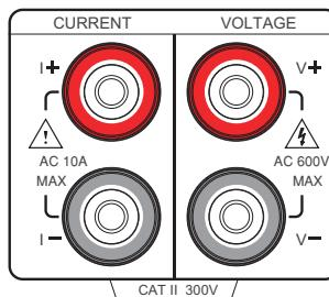
Current input: I+ and I- terminals; Voltage input: V+ and V- terminals.
