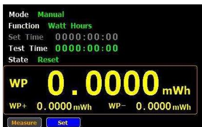
Standard mode    1. Set integrator measurement time before using integrator function.
