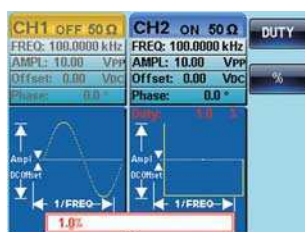
1% Duty Cycle of Square Wave
