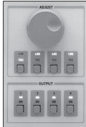
Up to four modules can be easily adjusted and controlled from the LDC-3900 front panel.
