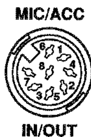
Figure A-1 MIC/ACC Connector Pin Identification
