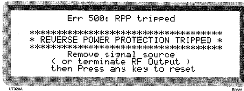
Fig. 4-16 RPP tripped display
